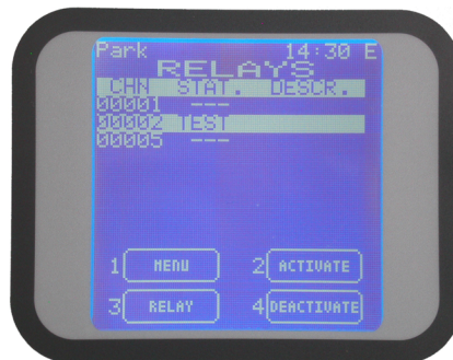
Figure 38) Output details screen in "Engineer" level
