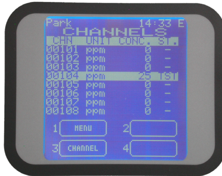
Figure 41) Screen with channel in "Test"
